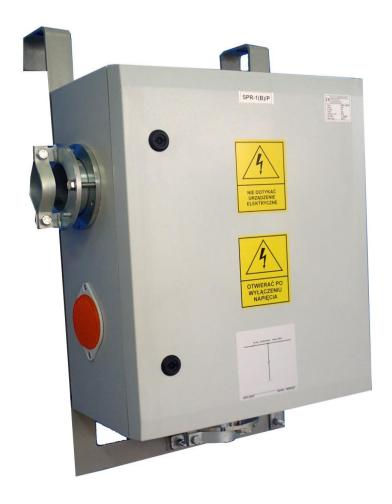
Switchgear type SPR-1(B)/P is an electrical device designed for use in the underground mining faces in non-explosive hazard conditions and on the ground in environment 2. Switchgear type SPR-1(B)/P is designed for connecting and branching-off mine 3-phase grid circuits with insulated star point of the transformer (IT system) for the grid rated voltage of 500V.
